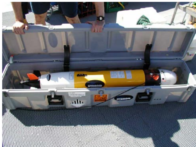
Figure 1: The REMUS in its Transportation Container
