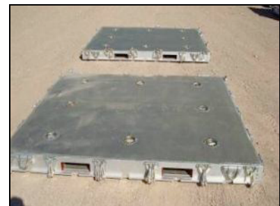
Figure 28. Post-drop Composite ECDS Platform
