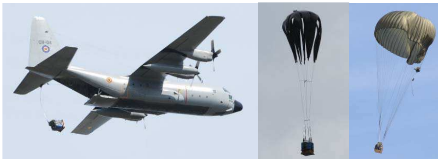
Figure 8: The BE C-130 drops a CDS / a HV-LCADS / AGAS steering
