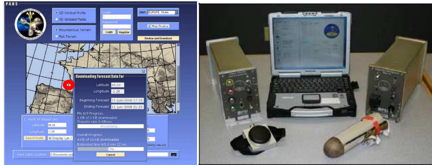
Figure 1: JAAWIN interface(Biscarosse : red circle) and JPADS-MP block III, including the drop sonde (below right).
