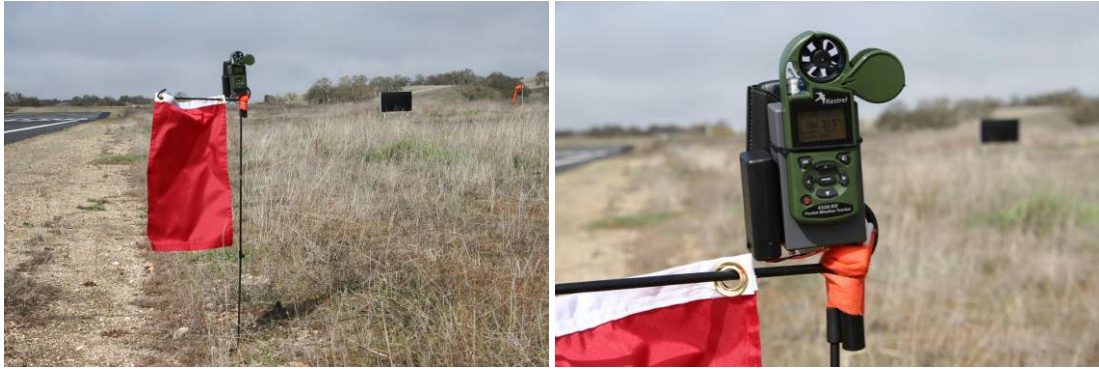
Fig. 12 Red target with a miniature wireless weather station and Blackberry phone.
