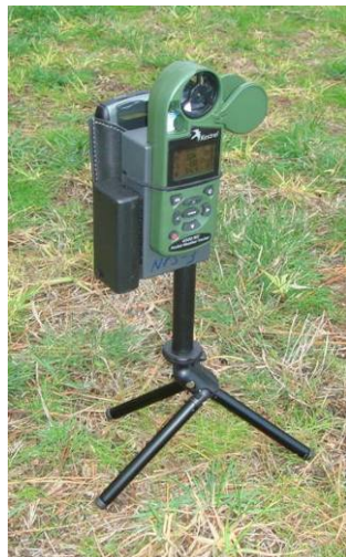
Fig. 7. The wireless target weather station posting its data over Blackberry handheld (on the back).
