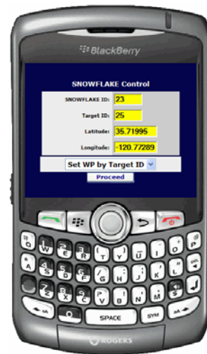
Fig. 8 Blackberry Curve 8310 handheld with Snowflake control interface.
