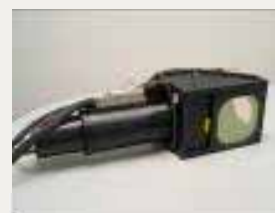
Lidar Leica ALS40 modified for profiling at altitude (12 km or more)
