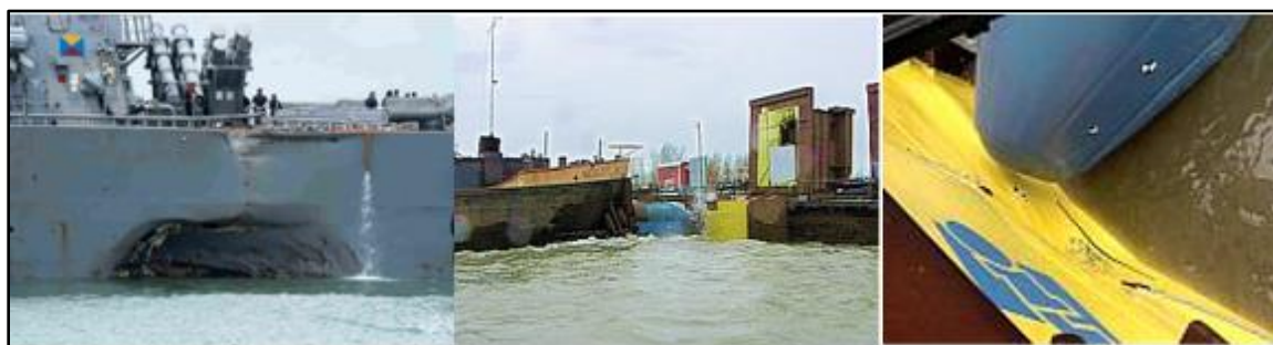
Figure 8. (left) Collision Damage to USS John S. McCain , August 2017; (center) Damen Shipyard Full-Scale Test (1998) of Collision-Resistant Ship Structure; (right) Structure Intact After Collision
