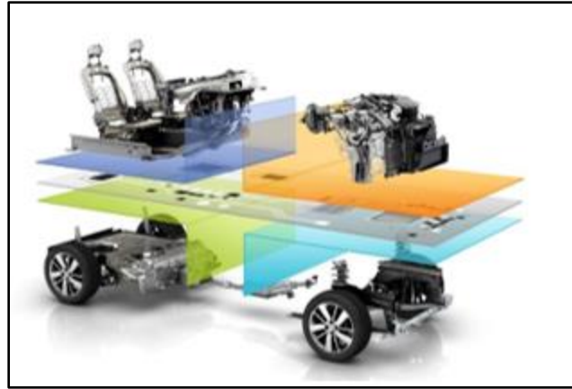
Figure 2. Automotive Example of Product Line Engineering and Payload/Platform Management the Renault-Nissan Common Module Framework
