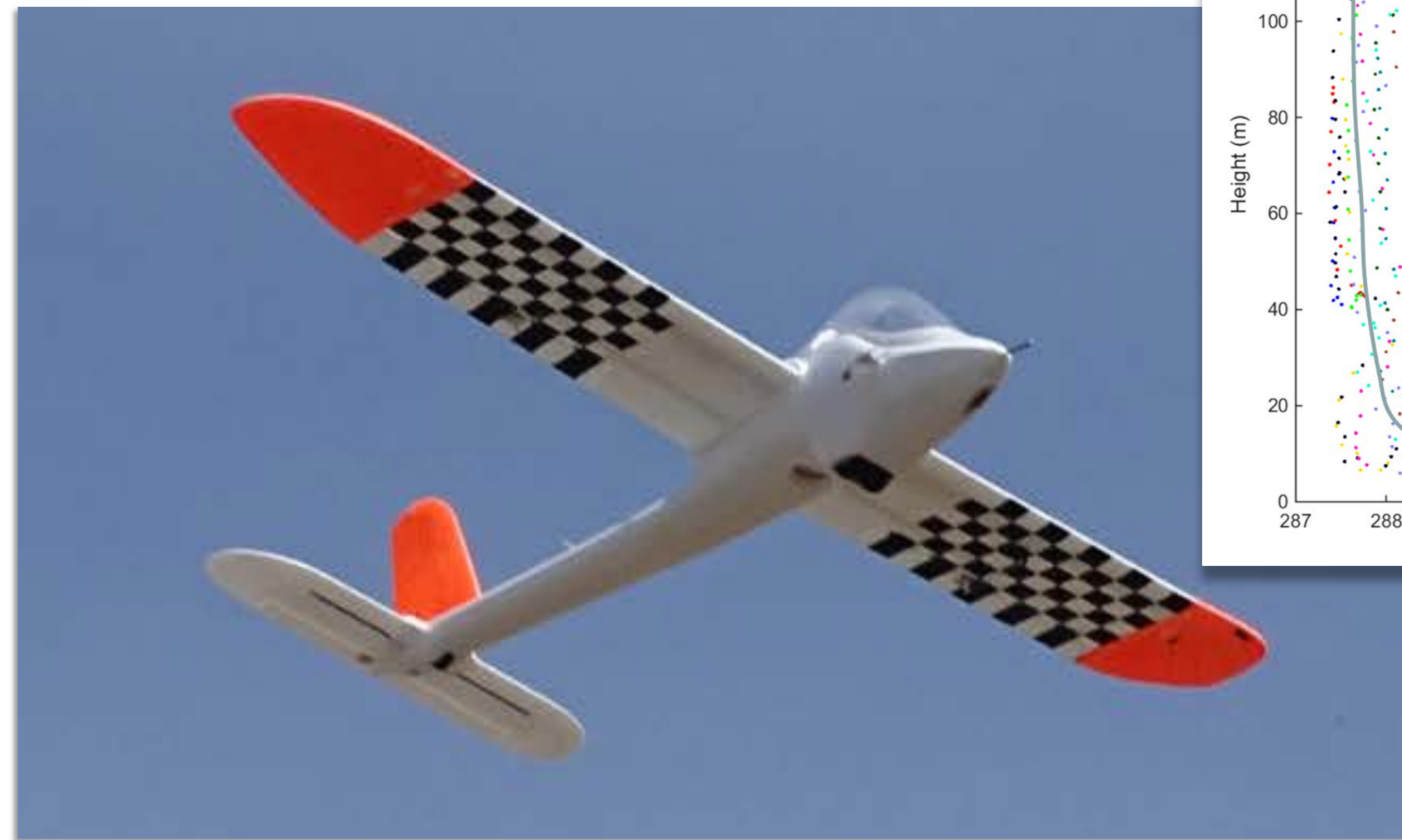
P-Met expendable UAS platform for sea-based low-cost near-surface meteorological sensing
