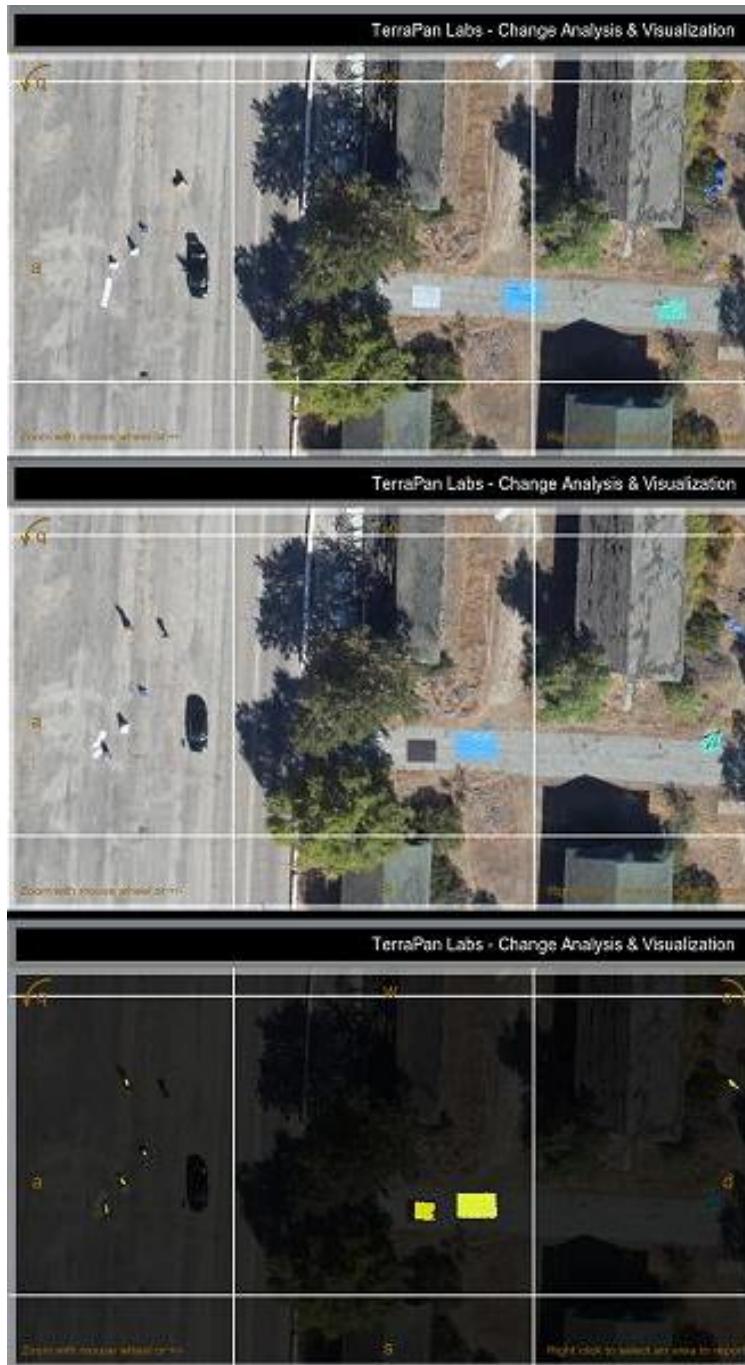
Figure 5. Change detection (top to bottom: first pass, second pass, change) example from repeat pass images collected Thursday August 16, 2012.
