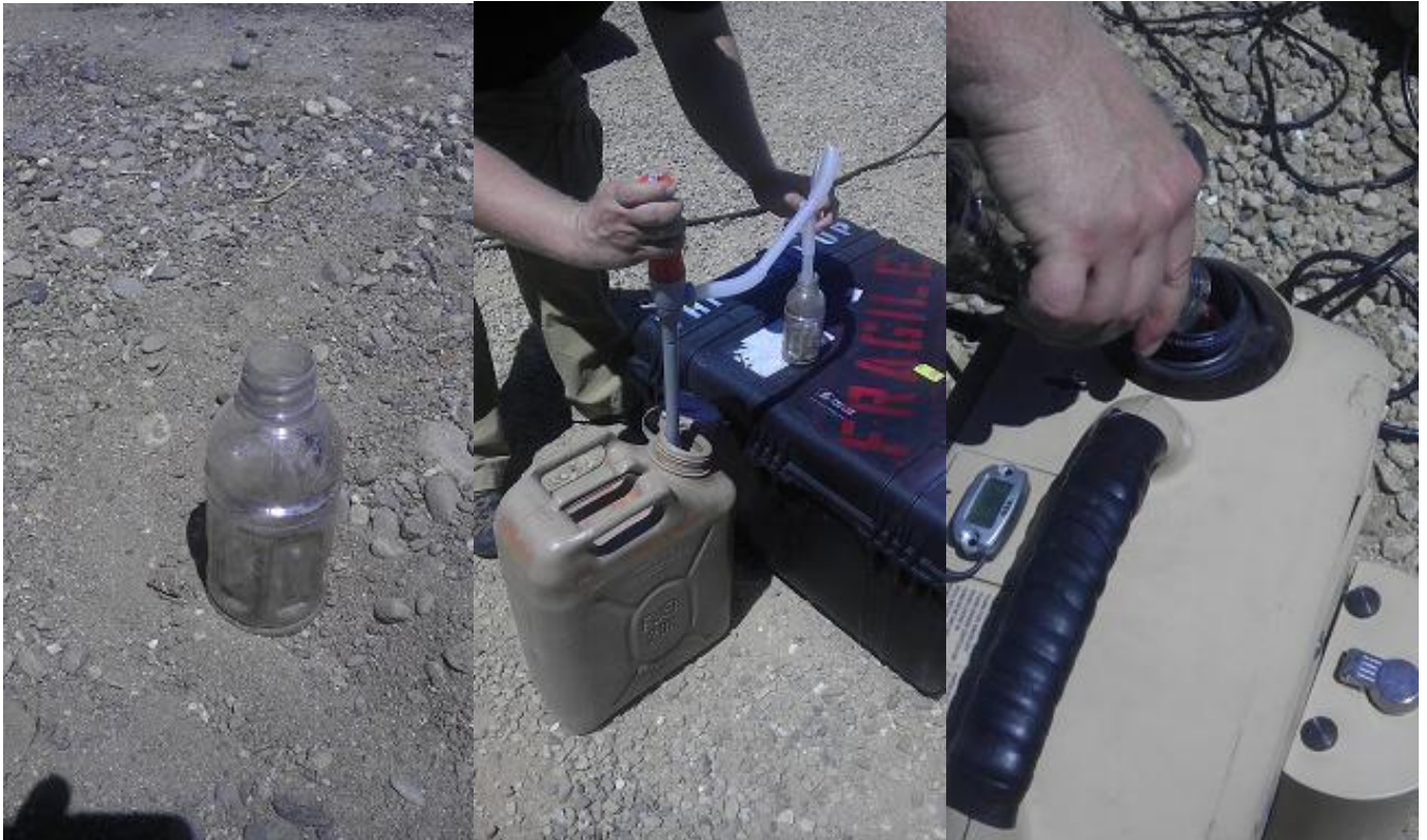
Left to right: Figure 4: Dirt added to container, Figure 3: Container then filled with JP-8, Figure 4: Successful operation on “Dirty JP-8” Pour
