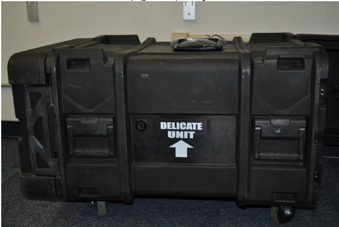
Figure 8. EOC in a box SKB shock case with removable front and rear doors and Cisco WAP.
