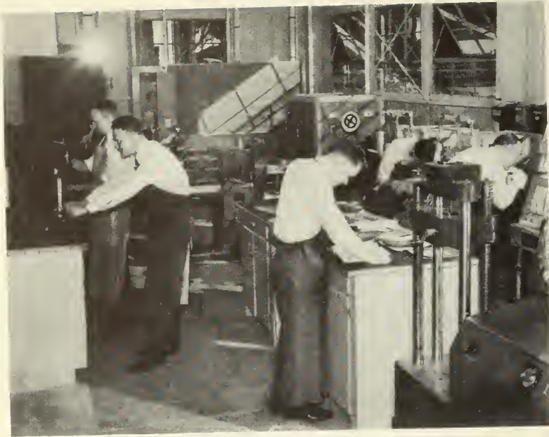
Metallurgy equipment, including hardness testers, rolling mill, furnaces and tension testing machine.
