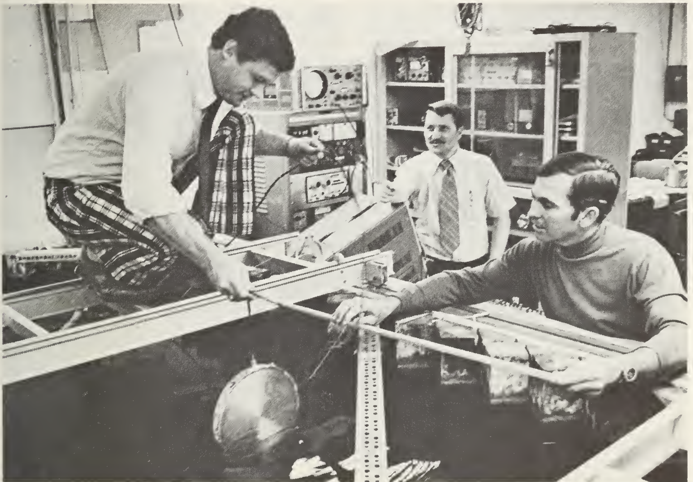
Students performing an acoustic experiment in an anechoic water tank.
