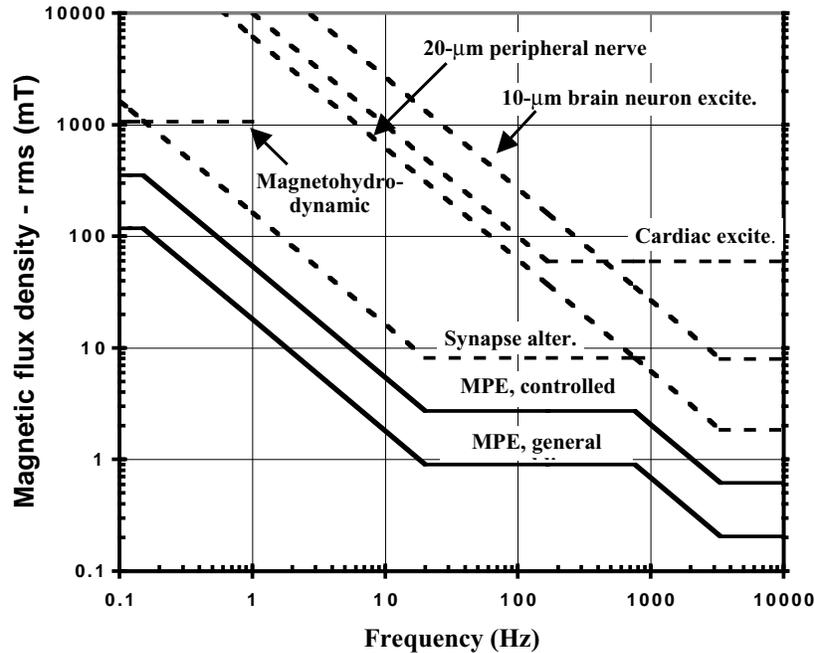
**Figure 1— Median thresholds for adverse stimulation from magnetic field exposure (broken lines) and recommended maximum permissible exposure limits (solid lines); whole-body exposure to spatially constant field**
