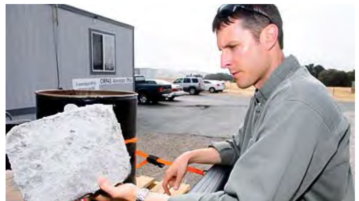
Former NPS student Lt. Deward Cummings holds a piece of light-weight, fibrous concrete while conducting thesis research into a recently-patented explosive containment technique. The effort is one of several NPS research projects completing the patent process in early 2016. (Courtesy photo)
