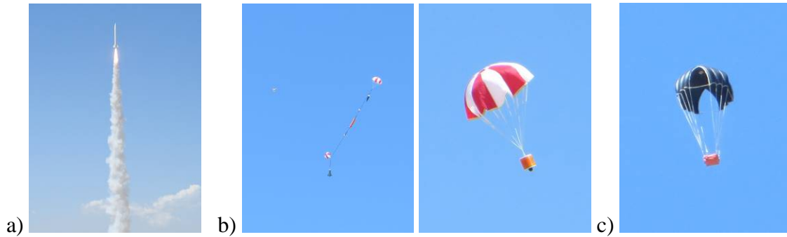
Figure 36. Rocket launch (a), second-stage UAS deployment (b), and steering cross-canopy (c).
