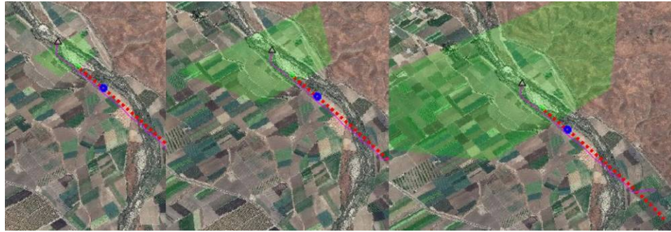
Figure 28. Onboard camera footprints with different zooms.
