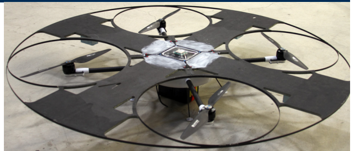
Flyable prototype with lower shell removed and feet attached
