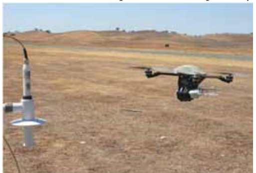
Figure 4. InstantEye UAV with Vaisala RS-92 radiosonde attached on bottom. The UAV is hovering next to a temperature/humidity sensor (left side) to verify and validate the UAV/radiosonde measurements.
